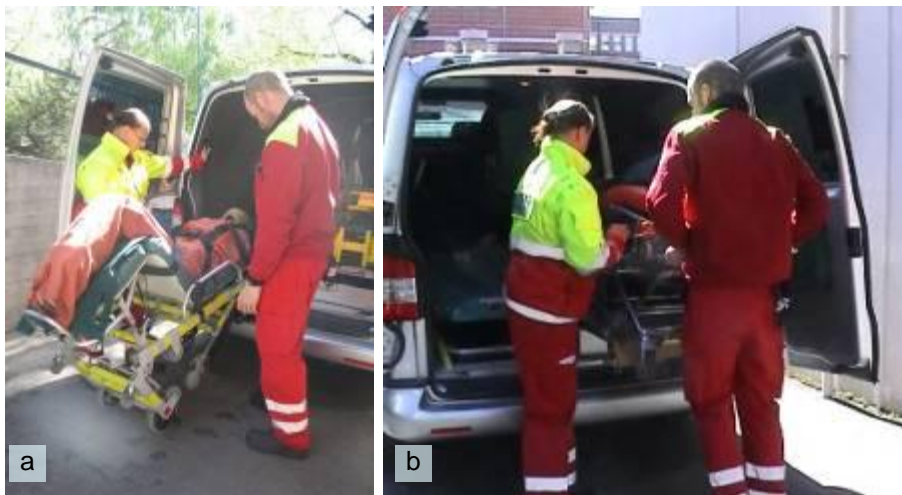
Figure 12. Loading the stretchers into the vehicle. a) Loading of the Pensi model is assisted by the Ergomy mechanism. b) The Ferno and Stryker models must be slid in along the loading ramp by lifting the foot of the stretcher.
