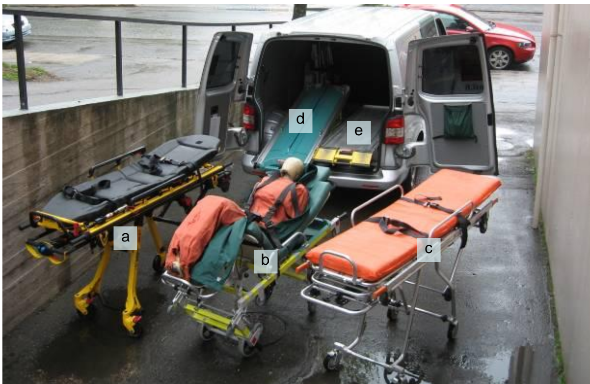
Figure 1. The stretchers included in the study: a) Stryker b) Pensi c) Ferno. The van with the required loading ramps installed can be seen in the background. d) Ergomy loading aid for the Pensi stretcher, e) loading ramp for the Ferno and Stryker stretchers.
