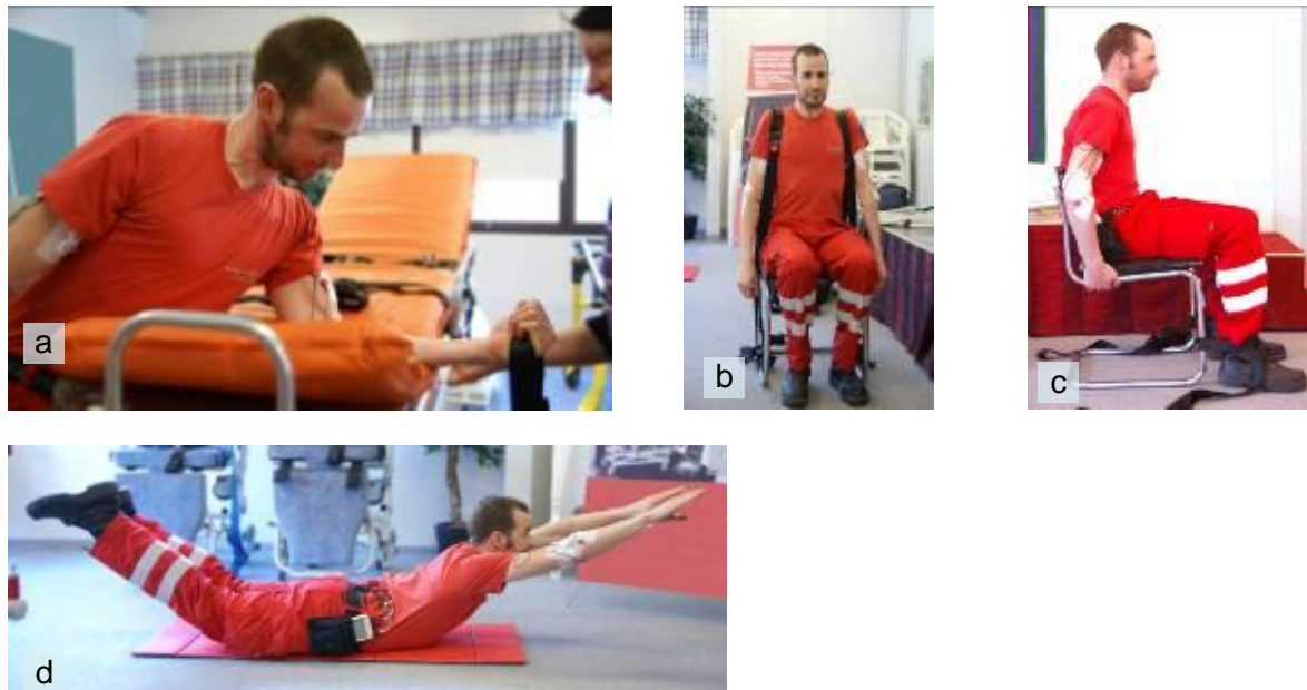
Figure 3. Calibration movements related to the electromyographic measurement, the purpose of which was to achieve maximal activation of the affected muscle group. a) Biceps and forearm b) Trapezius muscles c) Thigh (ankle attached to the chair leg with a strap) d) Low back muscles.
